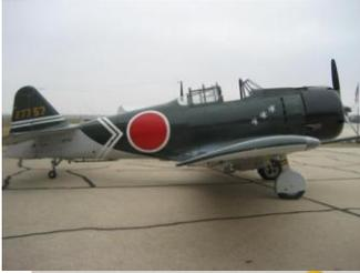
The windshield and upper deck were replaced, non-adjustable flaps added, slots cut in the fuselage side, wing tips reshaped using fibreglass, rudder profile changed and machine guns added.
